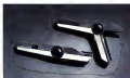
The early designs for the NES were sleek and cordless. The infrared components, it turned out, didn't work when moved around during game play.
